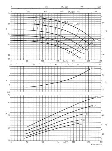
Type of slurry feed pump: KSB ETN 125-100-250
